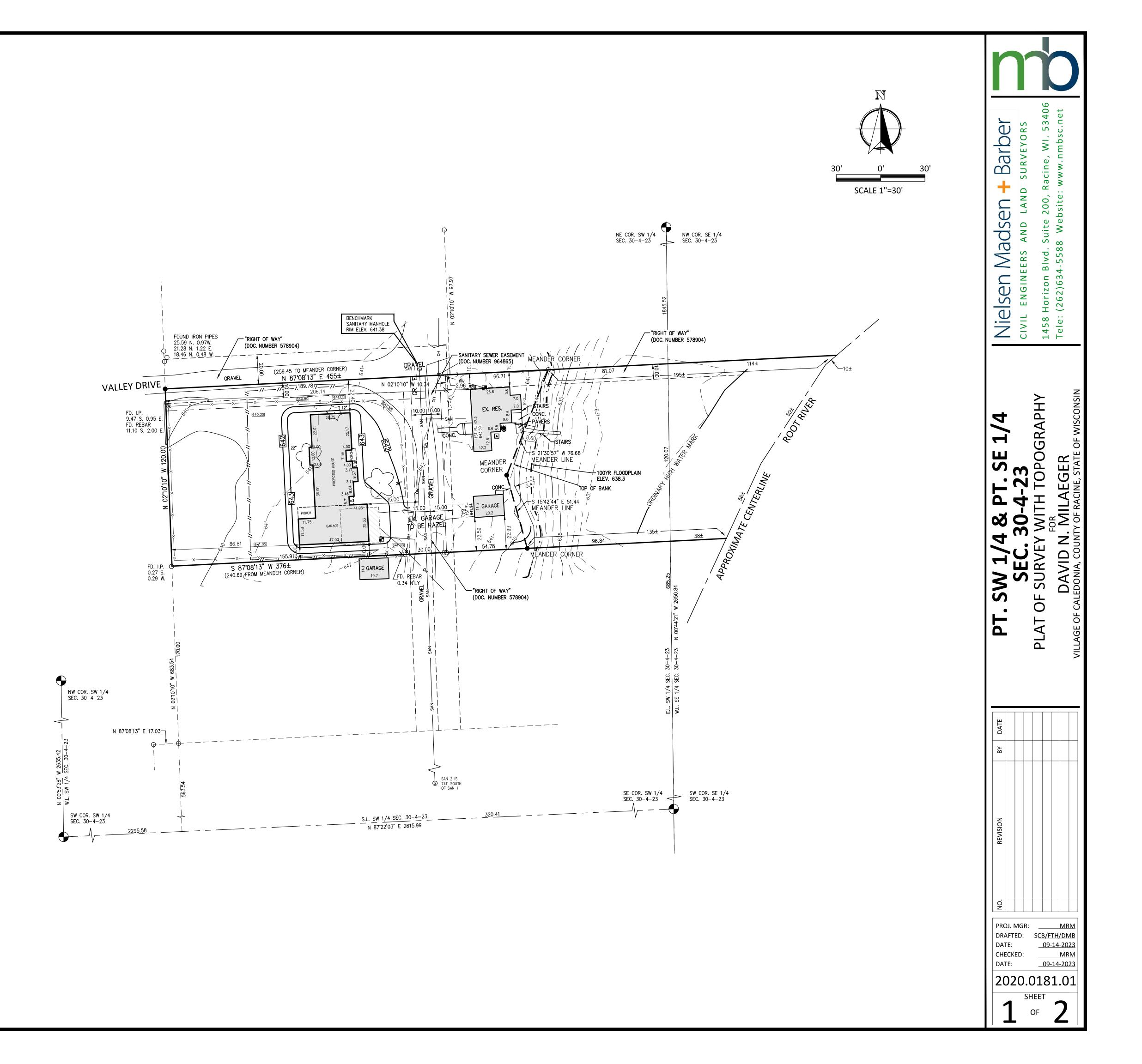
GRAVEL ACCESS DRIVE REQ'D. MIN 6" DEPTH, 2" TO 3" AGG. 10' WIDE X 35 L.F.
