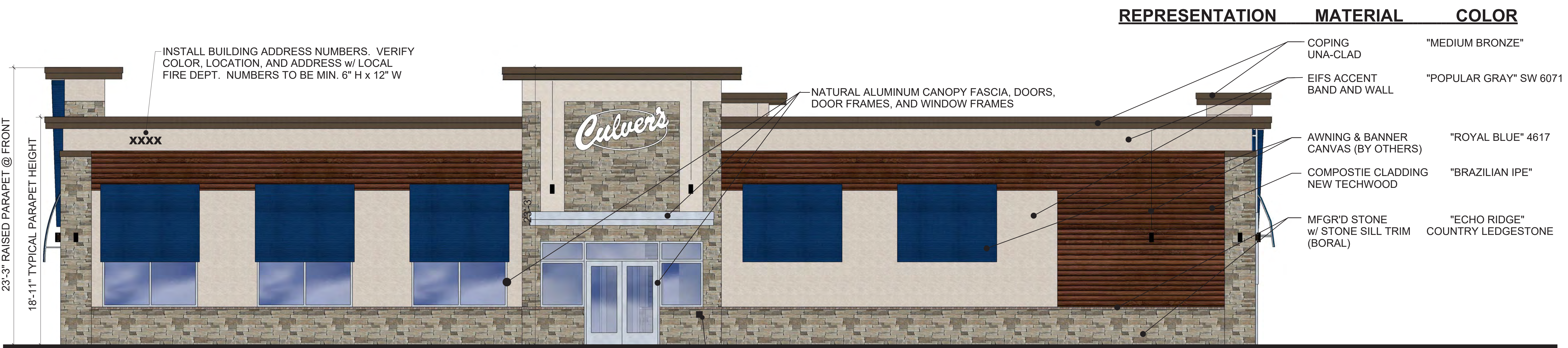
MAIN ENTRY ELEVATION
