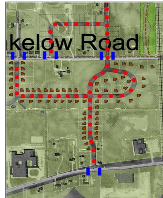
Figure 3-24. This diagram represents one conceptual site plan for Subarea E. This plan maintains critical access points and preserves a substantial amount of greenspace. For additional key symbols, see Page 39.
