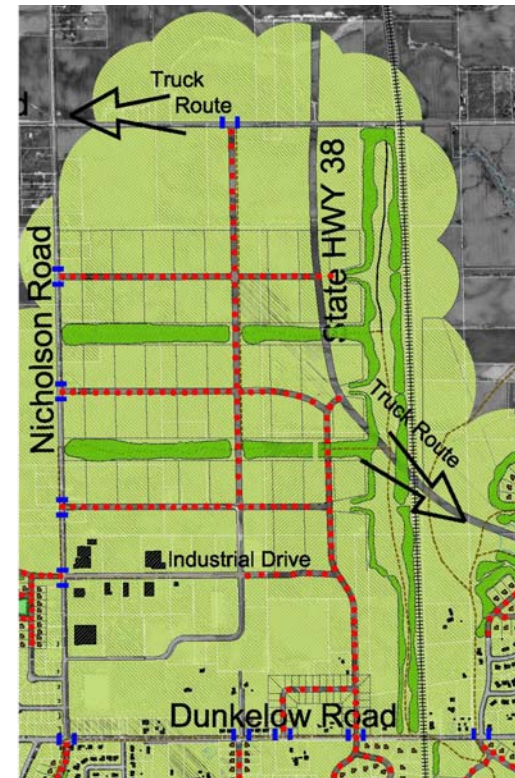
Figure 3-21. This diagram represents one conceptual site plan for Subarea D. This plan maintains critical access points. In order to deter industrial traffic from the residential areas, an access point is identified to the north and east, allowing a direct access to STH 38 and CTH K. An access point to Four Mile Road at the north is intended as a possible long range solution for moving industrial traffic to the interstate. This long term solution must be further investigated when additional areas of the industrial park are developed. For additional key symbols, see Page 39.
