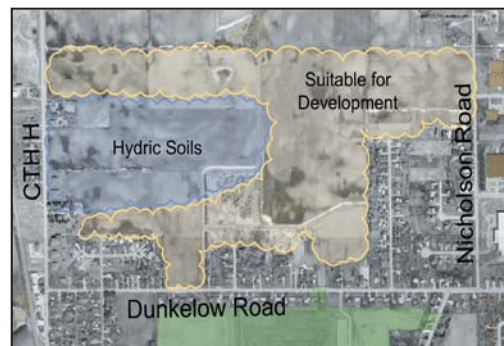
Figure 3-17. Diagrammatic illustration of soil conditions. Before any development occurs in this area, a detailed soils analysis must be completed.
