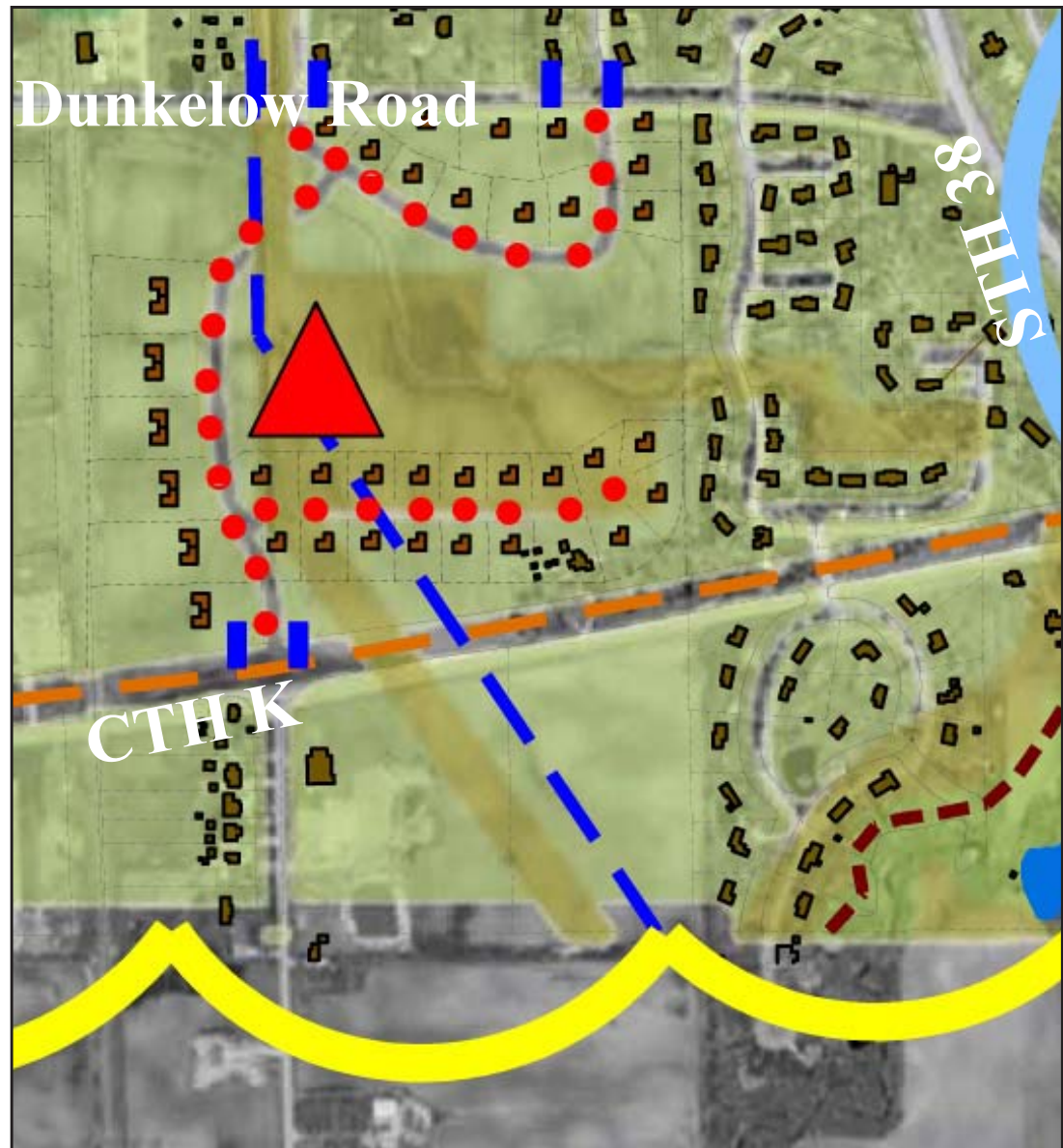
Figure 3-25. This diagram represents one conceptual site plan for Subarea F. This plan maintains critical access points and preserves a substantial amount of greenspace including land for a proposed park. For additional key symbols, see Page 39.
